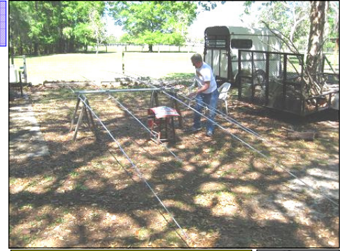
The antenna was assembled atop two sawhorses placed in the shade—thank goodness—in Cory's back yard. Note the shortness of the antenna's boom, only 8 feet
